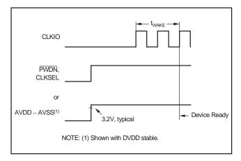
Figure 51. Device Wake Time with External Clock
