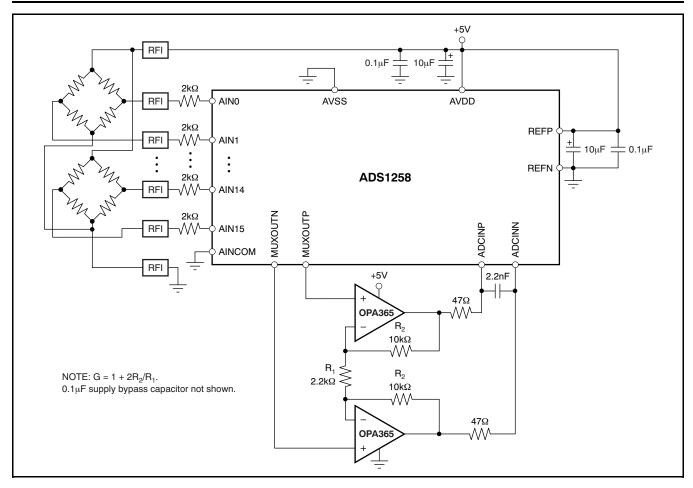
Figure 68. Bridge Input, Single-Supply Operation
