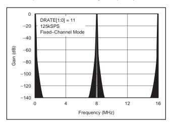
Figure 44. Frequency Response Out to 16MHz
