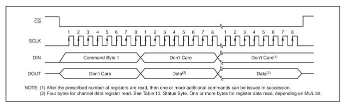
Figure 58. Register and Channel Data (Register Format) Read
