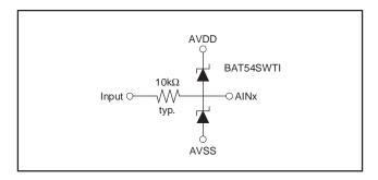
Figure 62. Input Overload Protection
