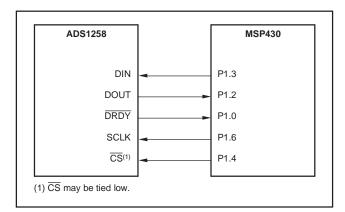
Figure 63. Connection to MSP430 Microcontroller
