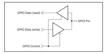
Figure 49. GPIO Port Pin
