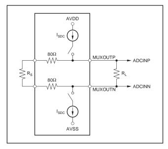
Figure 47. Sensor Bias Structure
