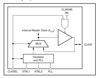
Figure 38. Clock Generation Block Diagram
