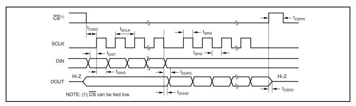
Figure 1. Serial Interface Timing
