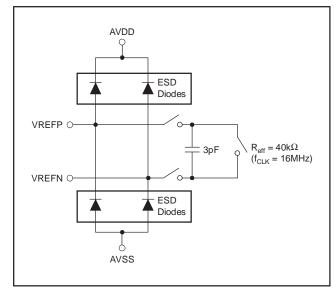
Figure 34. Simplified Reference Input Circuit
