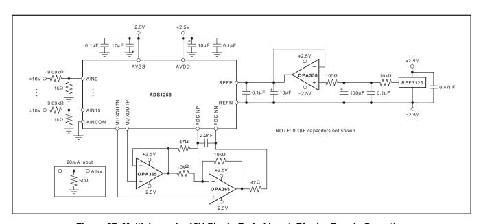
Figure 67. Multichannel, ±10V Single-Ended Input, Bipolar Supply Operation
