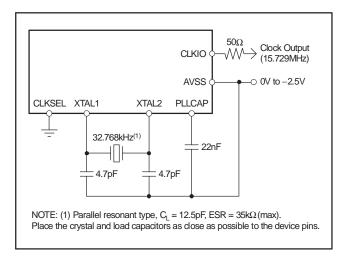
Figure 39. Crystal Oscillator Connection
