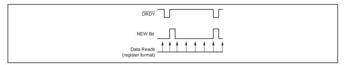
Figure 61. NEW Bit Operation
