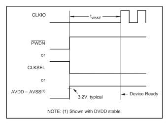
Figure 50. Device Wake Time with Internal Oscillator
