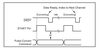
Figure 54. Pulse Conversion, Auto-Scan Mode
