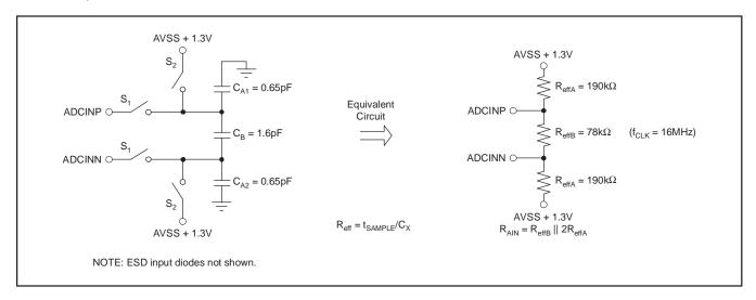
Figure 37. Simplified ADC Input Structure
