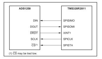
Figure 65. Connection to a TMS320R2811 DSP
