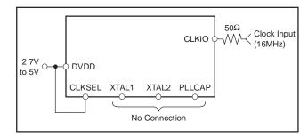
Figure 40. External Clock Connection
