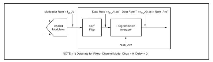
Figure 41. Block Diagram of Digital Filter
