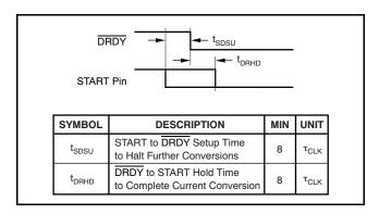
Figure 55. START Pin and DRDY Timing
