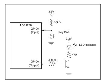
Figure 66. GPIO Connections
