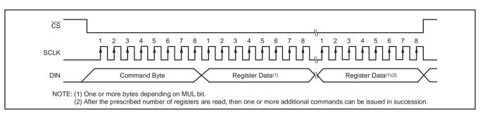
Figure 59. Register Write Operation
