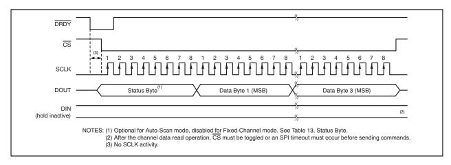
Figure 57. Channel Data Read Direct (No Command)
