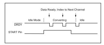
Figure 53. Conversion Control, Auto-Scan Mode
