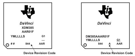
Figure 1. Example, Device Revision Codes (AAR Package)
