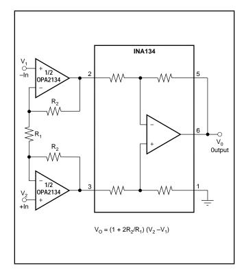
FIGURE 5. High Input Impedance Instrumentation Amplifier.
