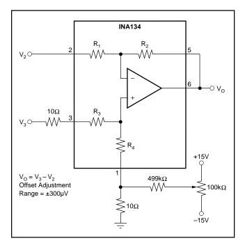
FIGURE 2. Offset Adjustment.
