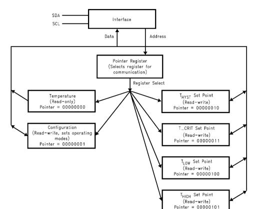
The data registers in the LM77 are selected by the Pointer register. At power-up the Pointer is set to "00"; the location for the Temperature Register. The Pointer register latches the last location it was set to. In Comparator Interrupt Mode, a read from the LM77 resets the INT output. Placing the device in Shutdown mode resets the INT and T\_CRIT\_A outputs. All registers are read and write, except the Temperature register which is read only.
