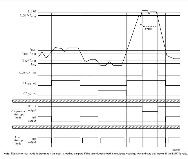
FIGURE 3. Temperature Response Diagram
