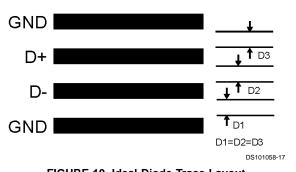
FIGURE 10. Ideal Diode Trace Layout
