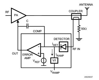
FIGURE 2. PA Control Loop
