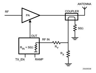
FIGURE 3. PA Control Loop With Extra Attenuation
