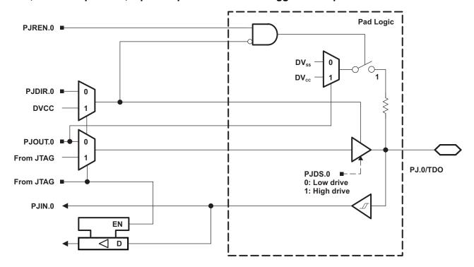
Port J, J.1 to J.3 JTAG pins TMS, TCK, TDI/TCLK, Input/Output With Schmitt Trigger or Output
