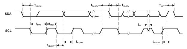
Figure 15. I2C Mode Timing
