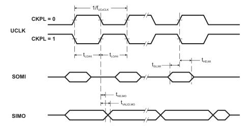
Figure 12. SPI Master Mode, CKPH = 1
