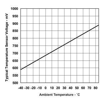
Figure 16. Typical Temperature Sensor Voltage
