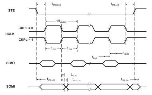
Figure 14. SPI Slave Mode, CKPH = 1
