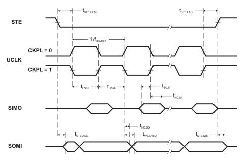
Figure 13. SPI Slave Mode, CKPH = 0
