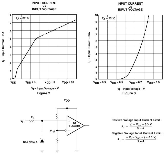
NOTE A: If the correct input state is required when the negative input exceeds GND, a Schottky clamp is required.
