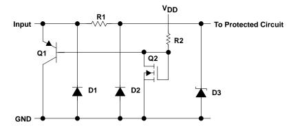
Figure 1. LinCMOS ESD-Protection Schematic
