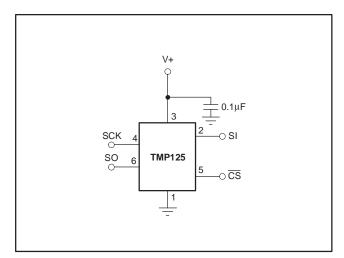
Figure 1. Typical Connections for the TMP125
