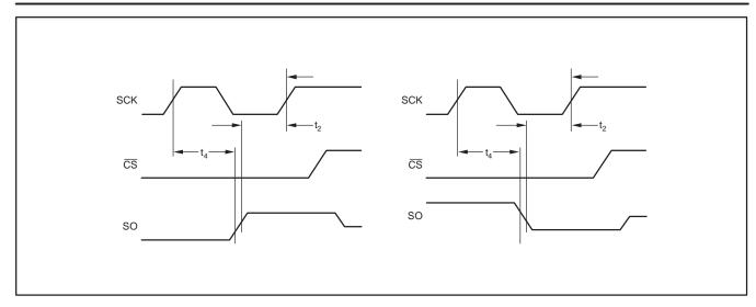
Figure 5. Input Data Timing Diagram
