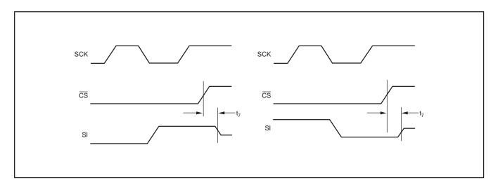
Figure 7. High Impedance Output Timing Diagram
