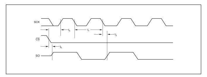
Figure 6. Output Data Timing Diagram
