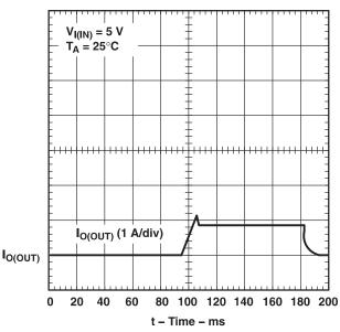
Figure 8. TPS2011A, Ramped Load on Enabled Device
