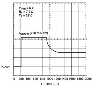
Figure 12. 7.9- $\Omega$  Load Connected to an Enabled TPS2010A Device
