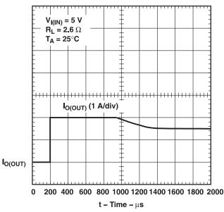
Figure 16. 2.6-Ω Load Connected to an Enabled TPS2012A Device
