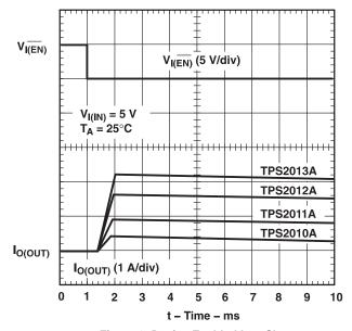
Figure 6. Device Enabled Into Short
