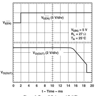
Figure 3. Turnoff Delay and Fall Time
