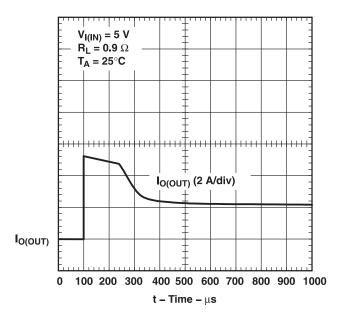
Figure 19. 0.9-Ω Load Connected to an Enabled TPS2013A Device
