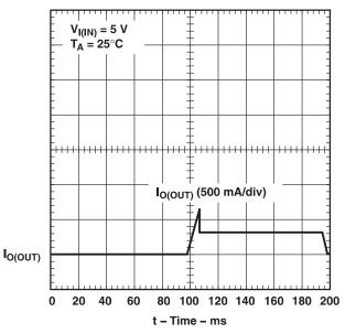
Figure 7. TPS2010A, Ramped Load on Enabled Device
