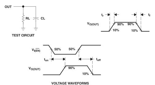
Figure 1. Test Circuit and Voltage Waveforms
