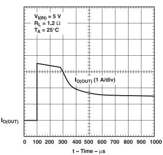
Figure 17. 1.2-Ω Load Connected to an Enabled TPS2012A Device
