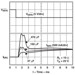
Figure 11. TPS2013A, Inrush Current
