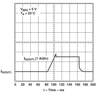
Figure 9. TPS2012A, Ramped Load on Enabled Device
