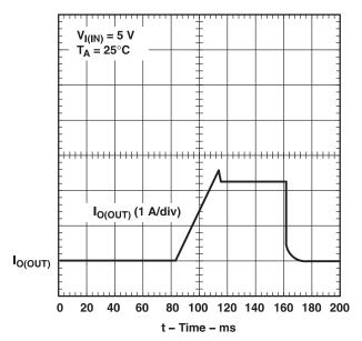
Figure 10. TPS2013A, Ramped Load on Enabled Device
