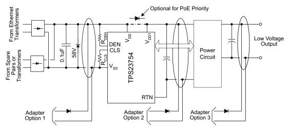
Figure 23. ORing Configurations
