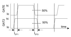
Figure 2. GATE and GAT2 Timing and Phasing
