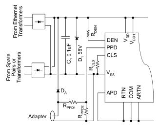
Figure 30. Low-Voltage Option 1 ORing
