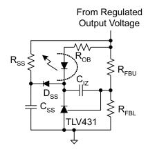
Figure 31. Error Amplifier Soft Start
