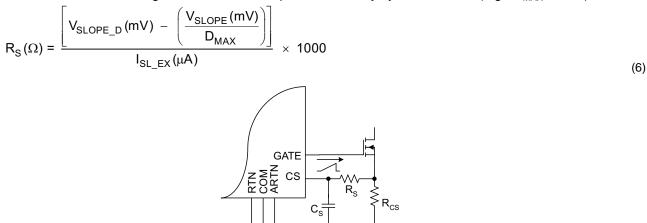
Figure 26. Additional Slope Compensation
