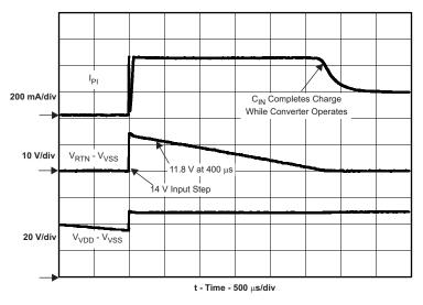
Figure 22. Response to PSE Step Voltage
