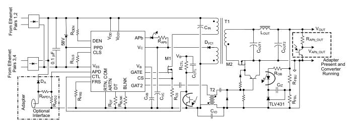
Figure 1. High Efficiency Converter Using TPS23757
