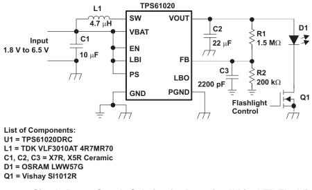
Figure 26. Simple Power Supply Solution for Powering White LED Flashlights
