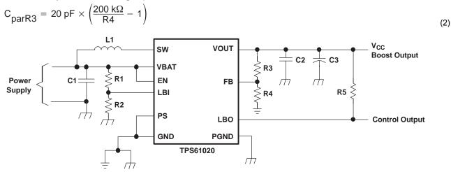
Figure 22. Typical Application Circuit for Adjustable Output Voltage Option
