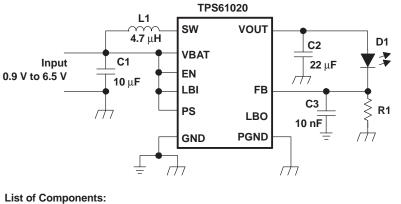
List of Components: U1 = TPS61020DRC L1 = Sumida CDRH2D16-4R7 C1, C2, C3 = X7R, X5R Ceramic D1 = White LED
