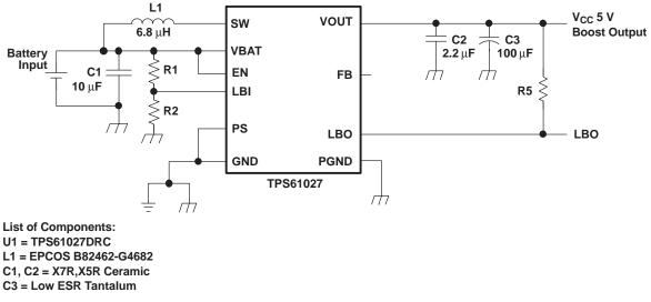
Figure 23. Power Supply Solution for Maximum Output Power Operating From a Single Alkaline Cell
