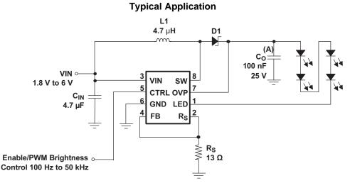
(A) Output capacitor values like 1 µF and larger, reduce the LED ripple current and improve line regulation.
