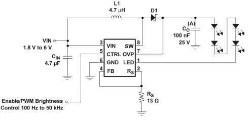
(A) Output capacitor values like 1 µF and larger, reduce the LED ripple current and improve line regulation.
