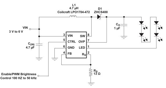
Figure 20. TPS61043 With 1-mm Total System Height
