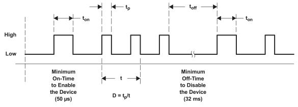
Figure 9. CTRL Timing Diagram
