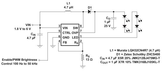
Figure 8. Schematic
