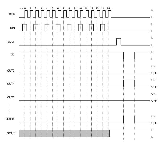
Note 1: The latch circuit is a leveled-latch circuit. Please exercise precaution as it is not triggered-latch circuit.
