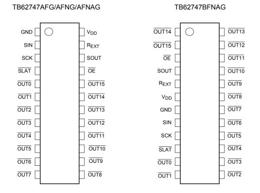
Note1: Short circuiting an output pin to a power supply pin (VDD or VLED\*), or short-circuiting the REXT pin to the GND pin will likely exceed the rating, which in turn may result in smoldering and/or permanent damage. Please keep this in mind when determining the wiring layout for the power supply and GND pins. \*VLED: LED power supply
