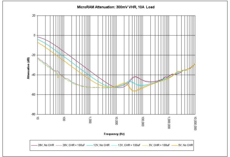
Figure 2 — MicroRAM attenuation with and without an additional CHR capacitor.
