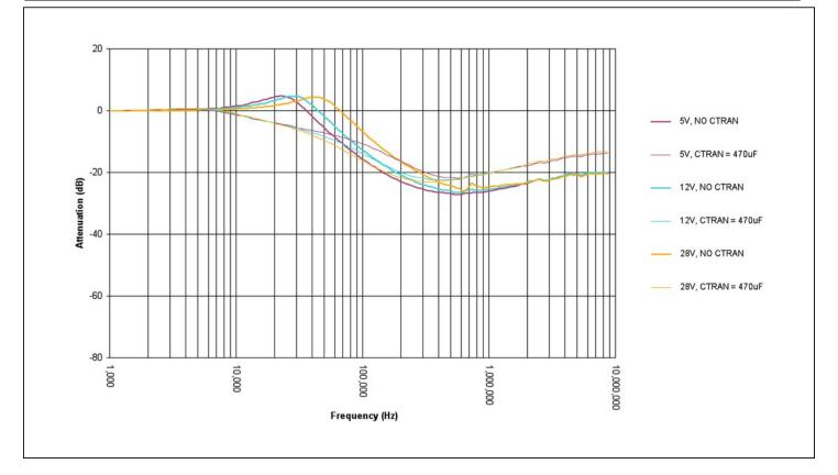
Figure 8 — MicroRAM's Passive Filter Attenuation with  $V_{HR}$  = 300 mV,  $I_{OUT}$  = 10 A
