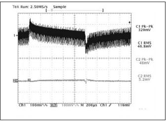
**Figure 24** — V300B12C250B and  $\mu$ RAM; Input and output dynamic response CTRAN = 820  $\mu$ F Electrolytic; 30% of load step of 6 A (10 A – 16 A); RHR = 80 k (Configured as in Figure 8 w/o Trim)
