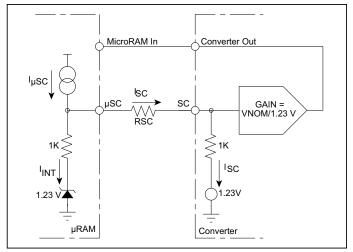
Figure 9 — MicroRAM's SC control circuit.
