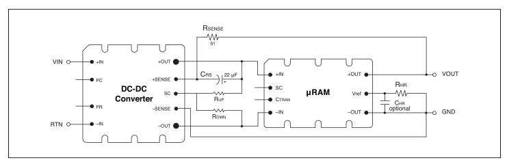
Figure 14 — Configuration for trimming a converter's output up/down using remote sensing.
