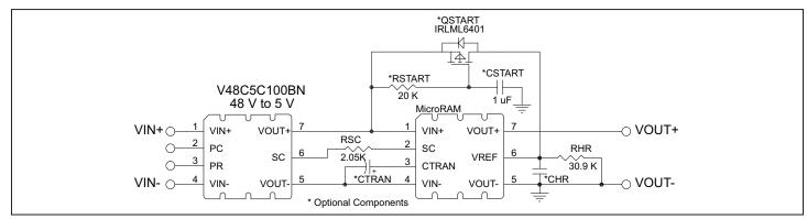
Figure 11 — Typical SC control configuration and an optional start-up circuit. R<sub>HR</sub> set for 375 mV of headroom voltage.
