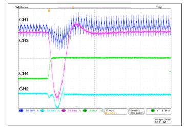
Figure 6 — Normal transient load response
