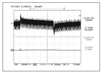
*Figure 23* — V300B12C250B and µRAM; Input and output dynamic response no added CTRAN; 17.5% of 20 A rating load step of 3.5 A (10 A – 13.5 A);RHR = 80 k (Configured as in Figure 7 w/o Trim)
