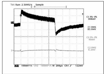
**Figure 21** — V375A28C600B and  $\mu$ RAM; Input and output dynamic response CTRAN=820  $\mu$ F Electrolytic; 32.5% of load step of 6.5 A (10 A – 16.5 A); RHR=178 k (Configured as in Figure 7 w/o Trim)
