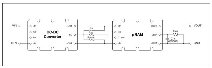
Figure 15 — Configuration for trimming a converter's output up/down using SC.
