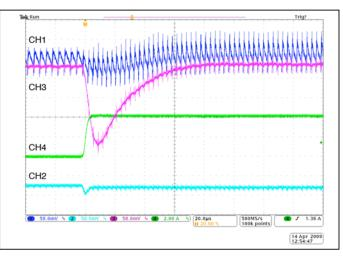
Figure 7 — Transient response with added CTRAN capacitor
