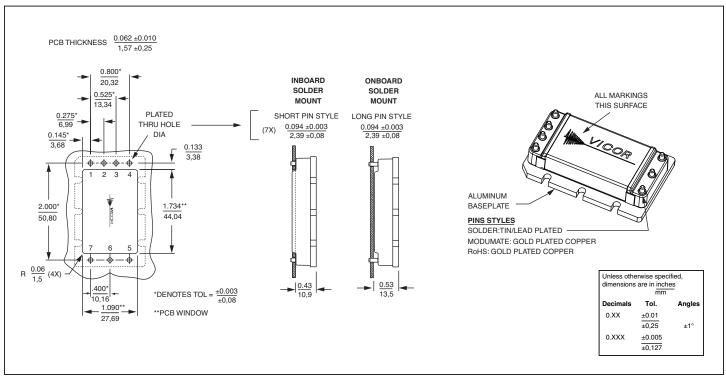
Figure 29 — PCB mounting specifications
