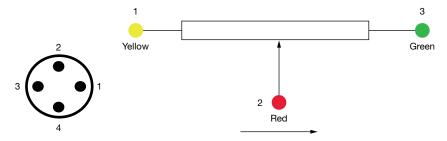
Direction of wiper displacement with shaft extended
