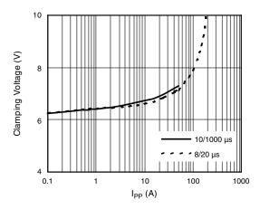
Fig. 4 - Clamping Voltage vs. Peak Pulse Current (T<sub>J</sub> initial = 25 °C)
