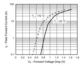
Fig. 7 - Typical Peak Forward Voltage Drop vs.
