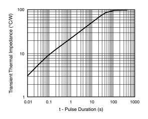
Fig. 6 - Typical Transient Thermal Impedance
