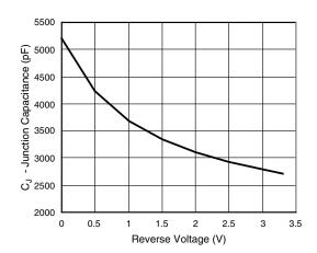
Fig. 5 - Typical Junction Capacitance
