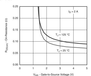
On-Resistance vs. Gate-to-Source Voltage
