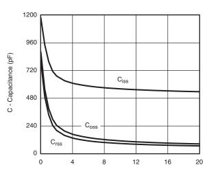
V<sub>DS</sub> - Drain-to-Source Voltage (V)
