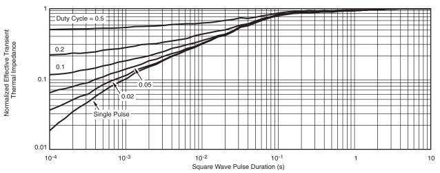
Normalized Thermal Transient Impedance, Junction-to-Foot
