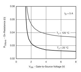
On-Resistance vs. Gate-to-Source Voltage
