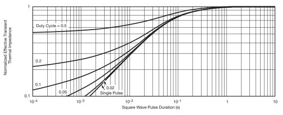
Normalized Thermal Transient Impedance, Junction-to-Foot
