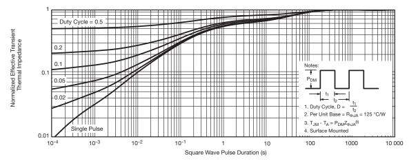
Normalized Thermal Transient Impedance, Junction-to-Ambient
