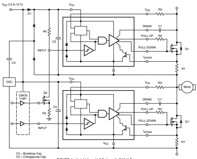
FIGURE 1. High-Voltage Half-Bridge with Si9910 Drivers
