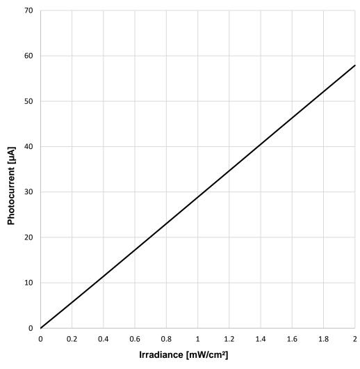
Testcondition: Ee=0,5mW/cm<sup>2</sup>, VR=5V
