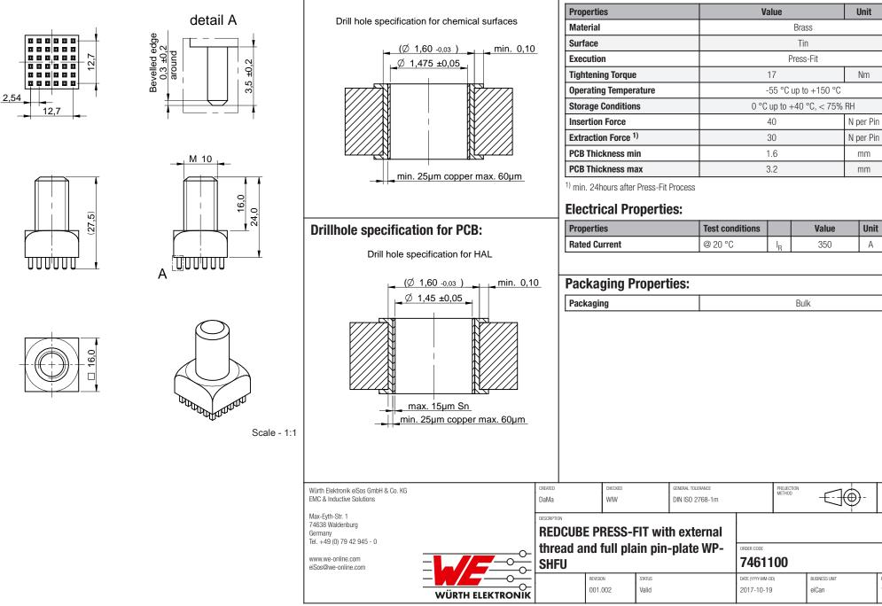
**Drillhole specification for PCB:**
