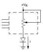
Two terminal Variable Resistor; Variable current
