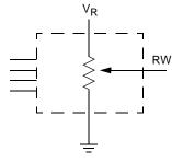
Three terminal Potentiometer; Variable voltage divider
