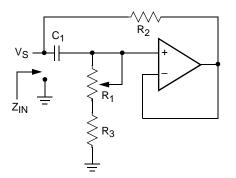
$\begin{array}{l} Z_{IN} = R_2 + s \; R_2 \; (R_1 + R_3) \; C_1 = R_2 + s \; \text{Leq} \\ (R_1 + R_3) >> R_2 \end{array}$
