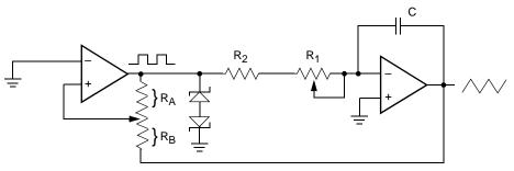
$\begin{array}{l} \mbox{frequency} \propto R_1,\,R_2,\,C \\ \mbox{amplitude} \propto R_A,\,R_B \end{array}$
