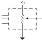
Three terminal Potentiometer; Variable voltage divider
