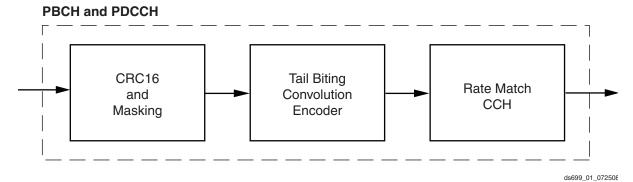
Figure 1: Downlink Channel Processing for BCH and DCI -CCH Channel Stream
