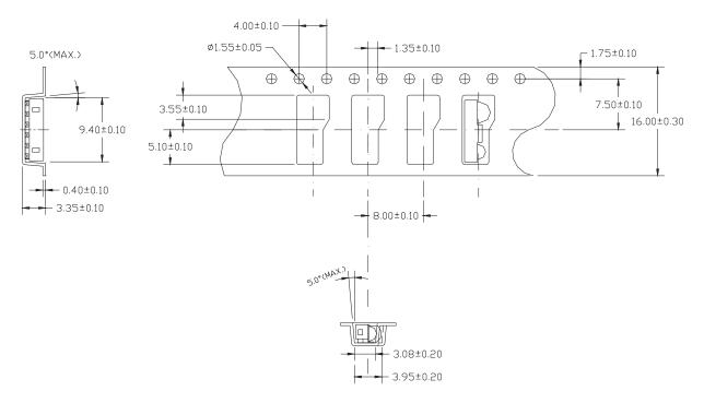
Figure 14. Alternative ZHX1810 Tape Dimensions and Configuration (Unit: mm) for Figure 9
