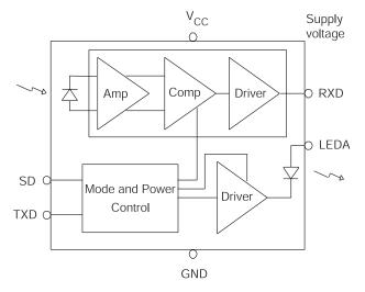
Figure 1. Slim SIR Transceiver Block Diagram
