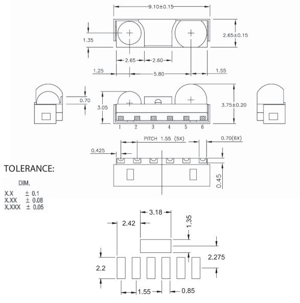
Figure 9. Alternative ZHX1810 Mechanical Drawing
