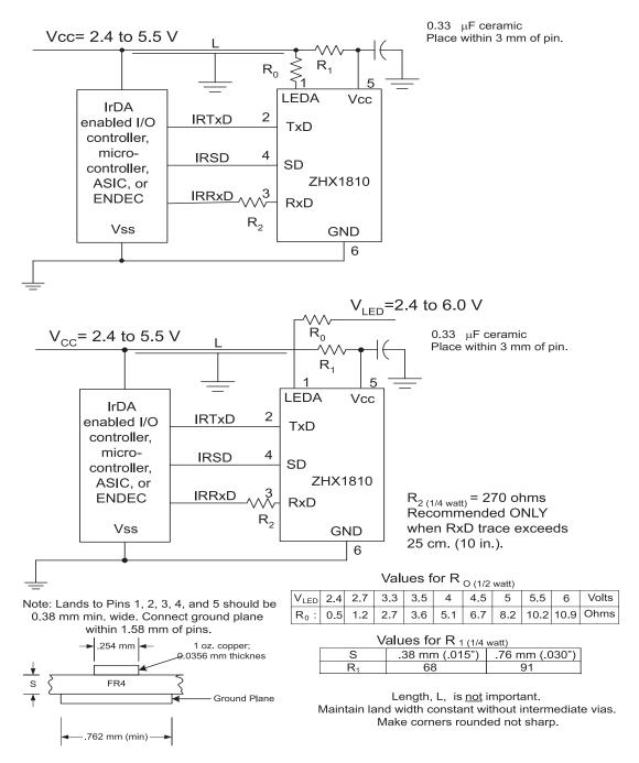
Figure 2. Application Block Diagrams
