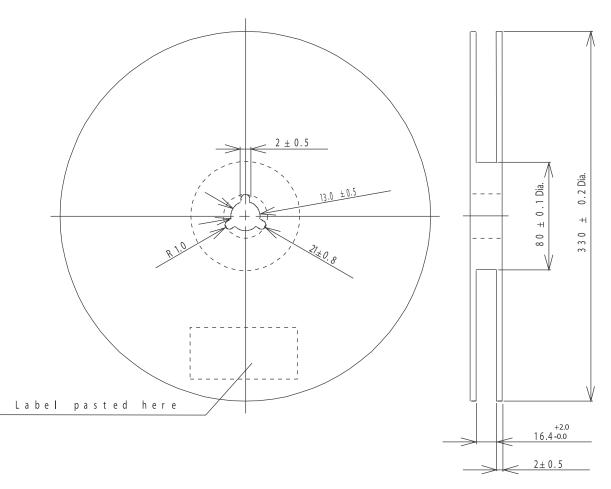
Figure 11. ZHX1810 Reel Dimensions (Unit: mm)
