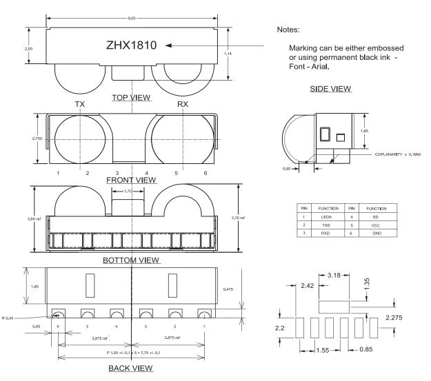
Figure 8. Alternative ZHX1810 Mechanical Drawing
