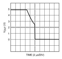
Figure 30. Output Signal With 20-pF Load
