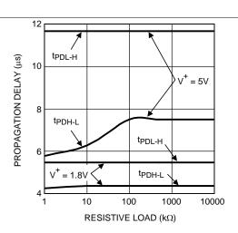
Figure 20. Propagation Delay vs Resistive Load
