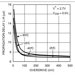
Figure 16. Propagation Delay vs Overdrive
