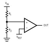
Figure 36. Threshold Detector
