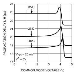
Figure 27. Propagation Delay vs Common-Mode Input
