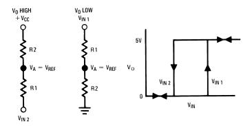
Figure 33. Noninverting Comparator With Hysteresis
