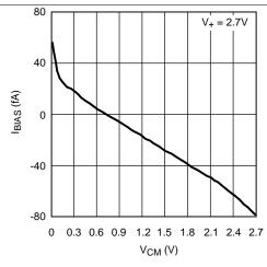
Figure 22.  $I_{\text{BIAS}}$  vs  $V_{\text{CM}}$
