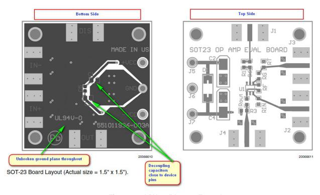
Figure 44. LPV7215 Layout Example
