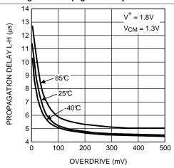
Figure 15. Propagation Delay vs Overdrive
