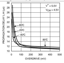
Figure 18. Propagation Delay vs Overdrive
