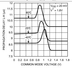
Figure 24. Propagation Delay vs Common-Mode Input
