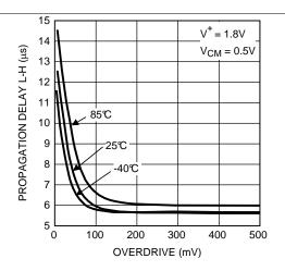
Figure 14. Propagation Delay vs Overdrive
