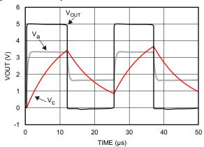
Figure 39. Square Wave Oscillator Output Waveform
