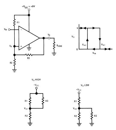
Figure 31. Inverting Comparator With Hysteresis
