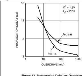
Figure 13. Propagation Delay vs Overdrive
