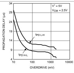
Figure 17. Propagation Delay vs Overdrive
