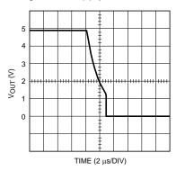
Figure 29. Output Signal Without Capacitive Load
