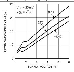
Figure 12. Propagation Delay vs Supply Voltage
