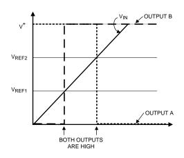
Figure 41. Window Detector Output Signal
