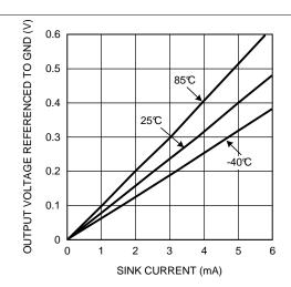
Figure 8. Output Voltage Low vs Sink Current
