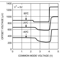
Figure 28. Offset Voltage vs Common-Mode Input
