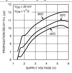
Figure 11. Propagation Delay vs Supply Voltage
