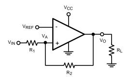
Figure 32. Noninverting Comparator With Hysteresis
