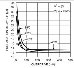
Figure 19. Propagation Delay vs Overdrive
