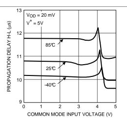
Figure 26. Propagation Delay vs Common-Mode Input
