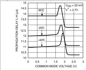
Figure 25. Propagation Delay vs Common-Mode Input
