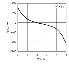
Figure 23.  $I_{BIAS}$  vs  $V_{CM}$
