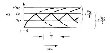
Figure 38. Square Wave Oscillator
