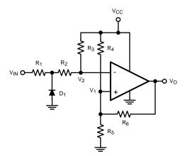
Figure 35. Zero Crossing Detector With Positive Feedback
