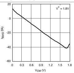
Figure 21.  $I_{\text{BIAS}}$  vs  $V_{\text{CM}}$
