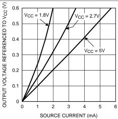
Figure 9. Output Voltage High vs Source Current
