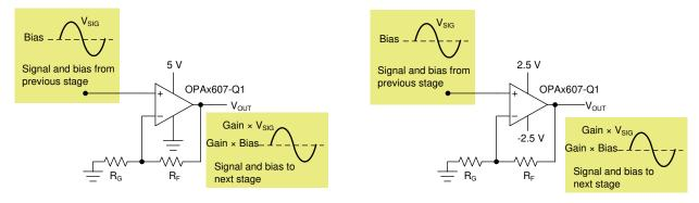
Figure 8-6. Single-Supply and Dual-Supply Operation
