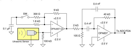
Figure 9-9. Hi-Z, High-Gain Front-End Circuit
