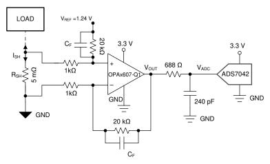
Figure 9-12. Low Side Current Sensing
