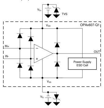
Figure 8-4. Internal ESD Structure
