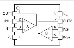
Figure 6-2. OPA2607-Q1 DGK 8-Pin, VSSOP Top View
