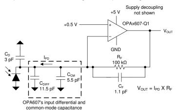
Figure 9-1. Wideband, High-Sensitivity, Transimpedance Amplifier
