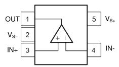
Figure 6-1. DBV Package 5-Pin SOT-23 Top View
