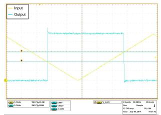
Figure 20. TLV3502 With Upper and Lower Threshold With 1-V Hysteresis
