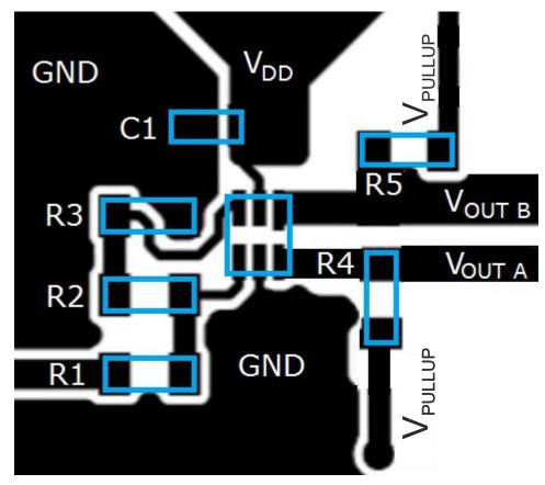
Figure 10-1. TPS3700-Q1 Layout Example
