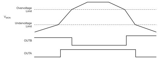
Figure 7-2. Window Voltage Detector Timing Diagram
