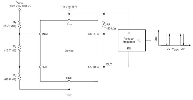
Figure 7-1. Window Voltage Detector Block Diagram
