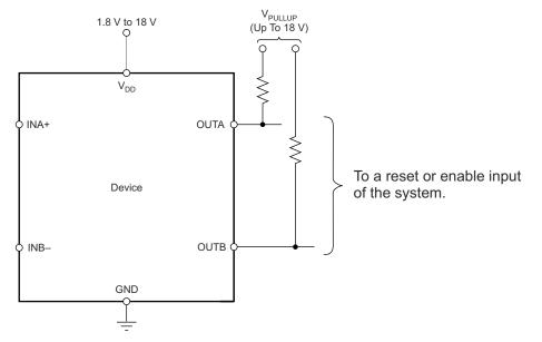
Figure 8-1. Interfacing to Voltages Other Than V<sub>DD</sub>
