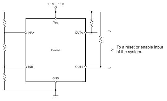
Figure 8-2. Monitoring the Same Voltage as V<sub>DD</sub>
