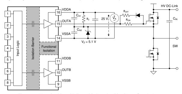
Figure 38. Negative Bias with Zener Diode on Iso-Bias Power Supply Output
