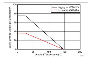
Figure 1. Thermal Derating Curve for Safety-Related
