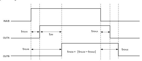
Figure 26. Overlapping Inputs, Dead Time Disabled
