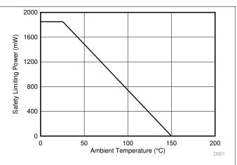
Figure 2. Thermal Derating Curve for Safety-Related Limiting Power
