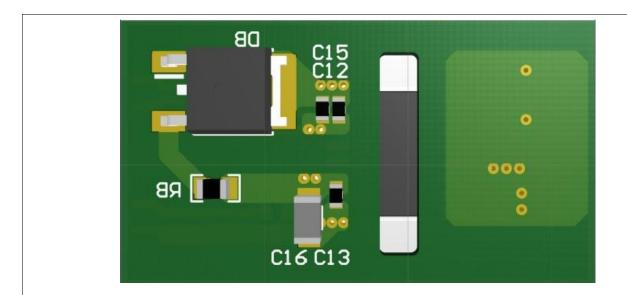
Figure 46. 3-D PCB Bottom View Showing Recommended Cutout
