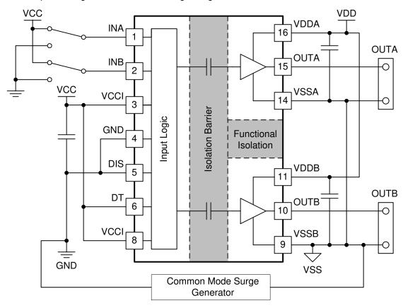
Figure 32. Simplified CMTI Testing Setup
