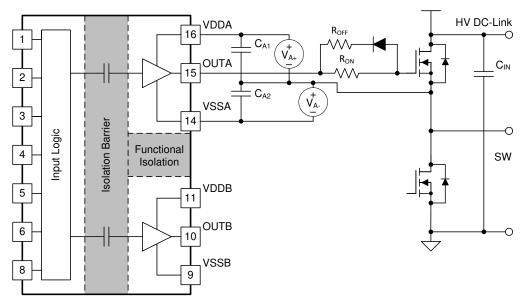
Figure 39. Negative Bias with Two Iso-Bias Power Supplies
