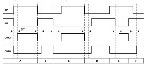
Figure 36. Input and Output Logic Relationship With Input Signals
