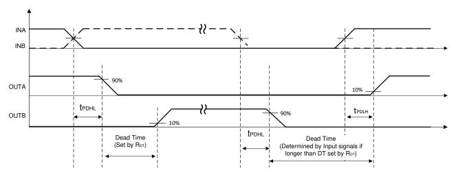
Figure 29. Dead-Time Switching Parameters
