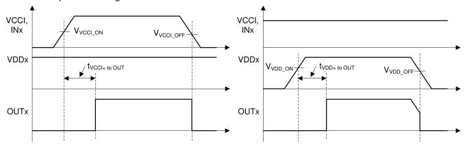
Figure 30. VCCI Power-up UVLO Delay
