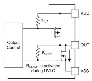
Figure 33. Simplified Representation of Active Pull Down Feature
