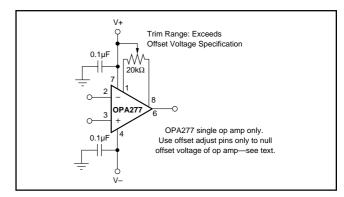
FIGURE 1. OPA277 Offset Voltage Trim Circuit.
