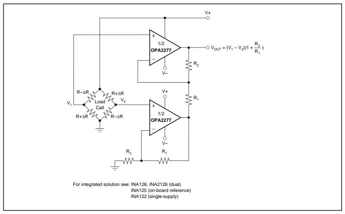
FIGURE 3. Load Cell Amplifier.
